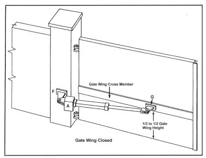
13. If both mounting brackets easily cover the marked outline, then mark through the bracket mounting holes in preparation for drilling and installation.
